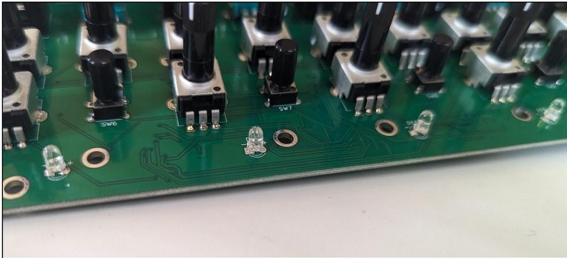
Attach and tighten all the Thonkiconn socket nuts, or at least those that are close to any LEDs and the 5-pin headers (J5-J6). **This ensures a constant distance between PCB and front panel which is important for soldering the LEDs and 5-pin headers.**
