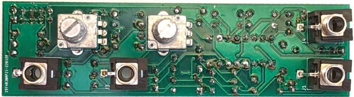
Remove the nuts from the pots (RV1, RV2) and jacks (J1-J4). You may want to clip the little silver anti-rotation tag off the pots with a wirecutter. Fit the pots and jacks onto the PCB without soldering yet. Then put on the front panel. Add and lightly tighten all the nuts to hold the panel in place. Carefully flip everything back over and solder.
