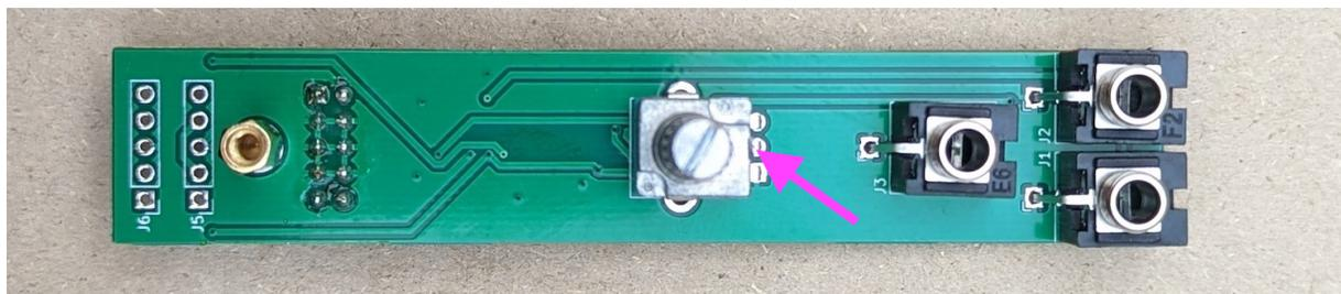
Snip off the little anti-rotation tab near the bottom of RV1 with a wirecutter. Put RV1 as well as J1, J2 and J3 in their places as shown. Put on the front panel, attach and lightly tighten the nuts to RV1 and the sockets. Solder all on the backside.
