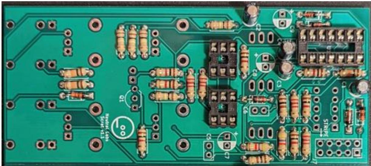
Put in the  $0.1 \mu\text{F}$  capacitors now (C1-C4). **Caution! Polarity matters for all of the electrolytic capacitors.** Their longer leg goes on the plus side as indicated on the PCB.
