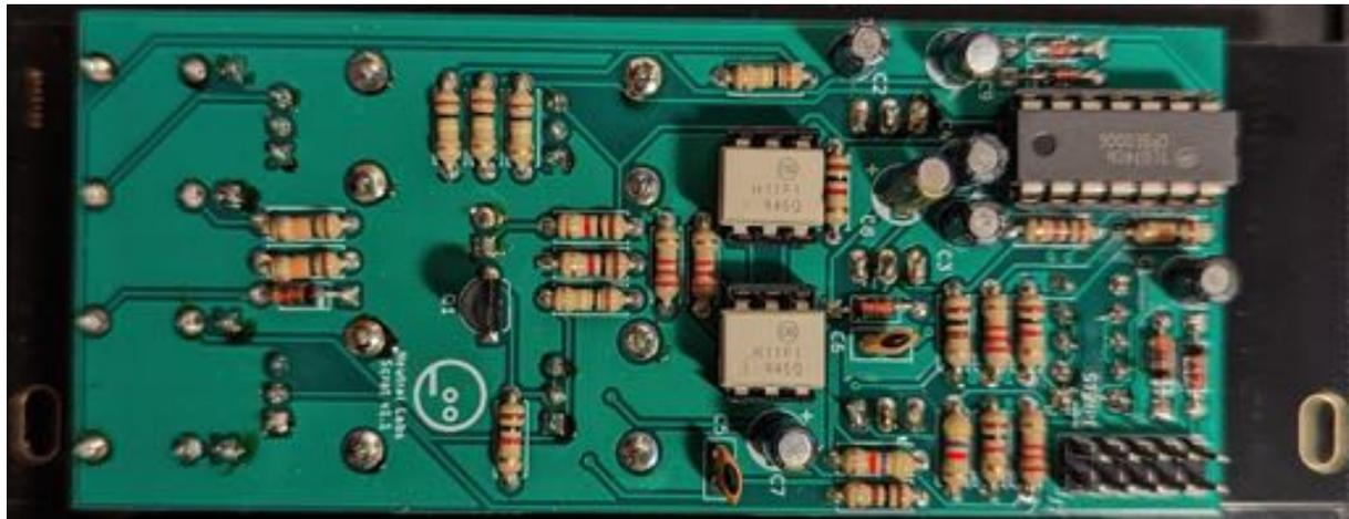
Plug the ICs into their sockets (U1 and OK1-OK2). They have little notches or dots on them, which should match the little notch on the socket (and the notch in the white outline on the PCB). Bend their legs slightly inward if you have trouble fitting them in.
