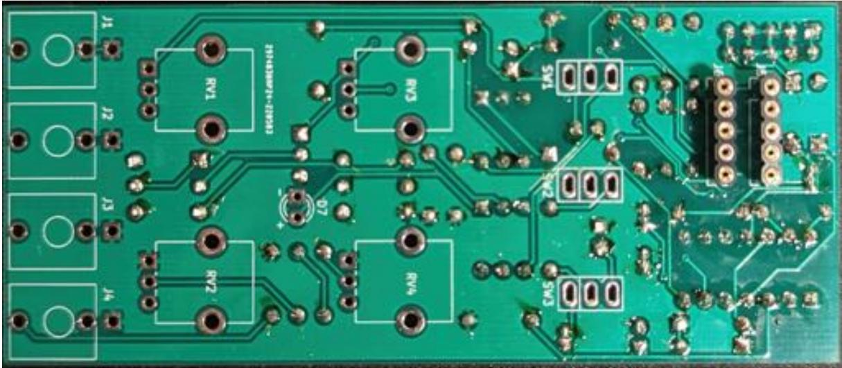
Flip the PCB over. Now on to J5 and J6 (the panel port headers). There are 2 different types of DIY kits with different types of headers. If your kit has headers with long legs that look like this, skip the next step.
