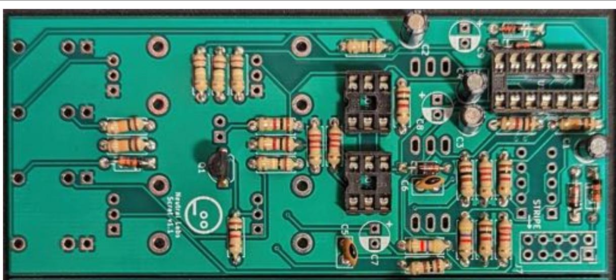
Put in the small 3.3 nF capacitors next (C5-C6, polarity does not matter for them). In your kit, C5 and C6 may be different in size, shape and/or color from the ones shown here. Don't worry, ceramic capacitors come in different designs, but they work the same way.
