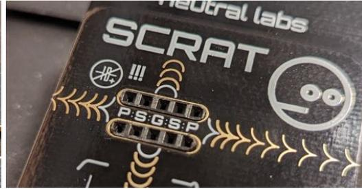
In case your kit has these 5-pin precision headers, it will also have a regular 19-pin or 20-pin female header strip (with short legs). Otherwise it will have two 5-pin headers with long legs.
