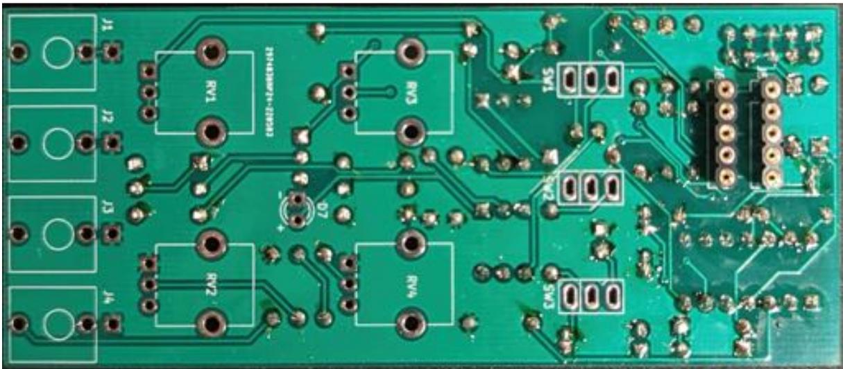
If your kit has two 5-pin precision headers with round holes and short legs, put them into J5 and J6 as shown and solder them. They are there in order to increase the overall height, so the panel port headers will be flush with the front panel.
