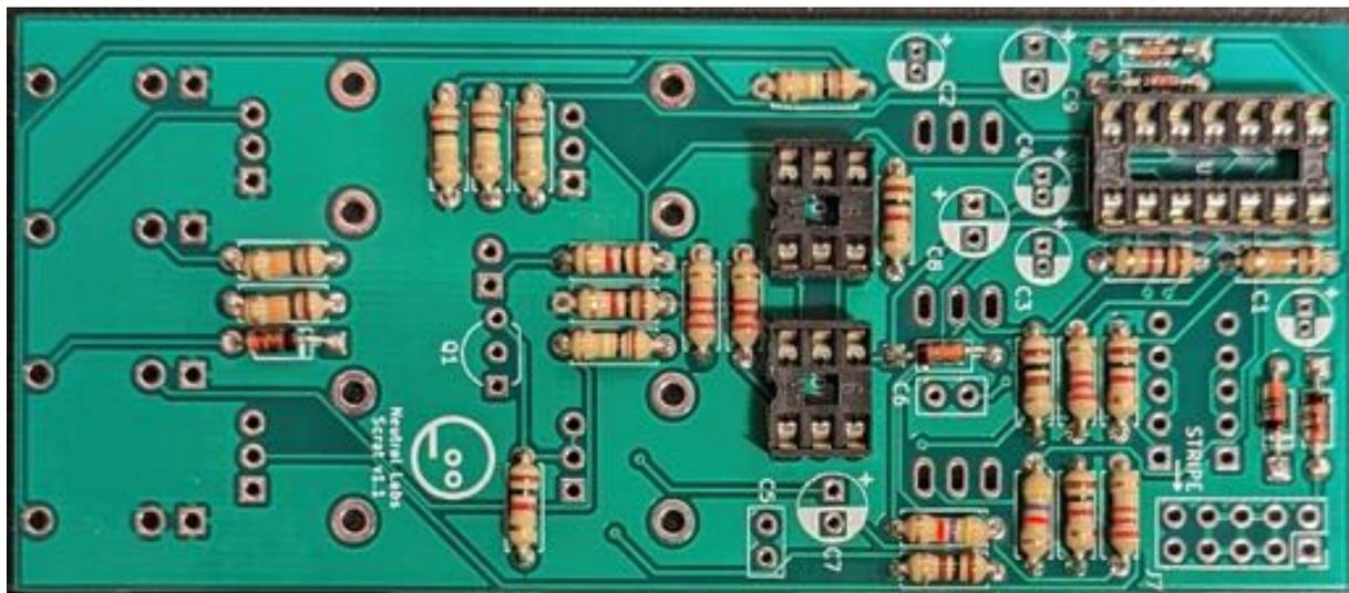
Next, put in the IC sockets (U1 and OK1-OK2). They have a little notch on one side which should match the notch of the white outline on the PCB. (It's not harmful if you put one in the other way around by accident, as long as you make sure the IC is facing the right way when you plug it in later.)
