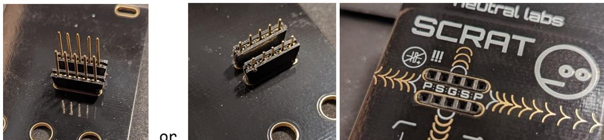
In case your kit has these 5-pin precision headers, it will also have a regular 19-pin or 20-pin female header strip (with short legs). Otherwise it will have two 5-pin headers with long legs.
