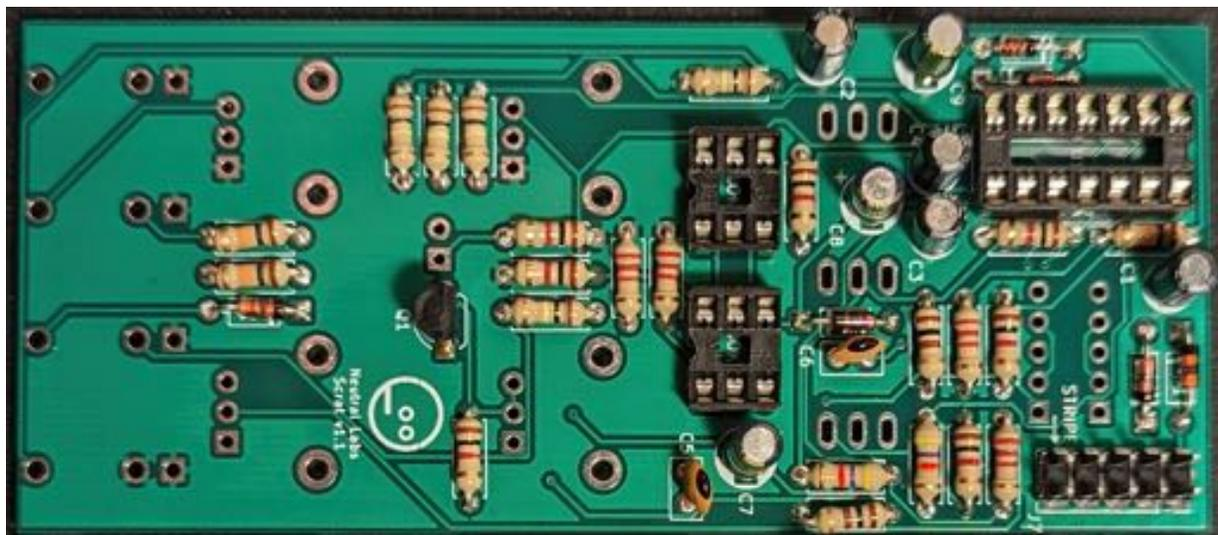
Now add the 10  $\mu$ F capacitors (C7-C9). **Caution! Polarity matters for C7-C9!** Put in the 2x5 pin power header (J7). As with the IC socket, it's best to solder a single pin first. You may want to hold the headers in place with a piece of sticky tape while soldering. Another trick is to plug the Eurorack power cable into the header before and hold it this way.
