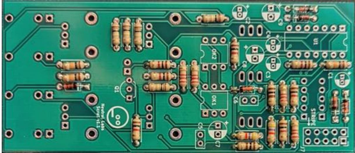
Solder the diodes D1-D6 (except D7!) and all resistors first (R1-R23). You do NOT have to read ring codes or use a multimeter to determine the resistor values. Neither do you have to use a loupe to inspect the labels on the diodes. There are only unique sets, so you can just count the ones in each set to find out the value. Some of the resistors in your kit may be white, green or blue instead of beige. Don't worry, they all work pretty much the same.
