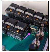
The short leg goes on the "-" side. This side is also marked with a stripe on the capacitor body. The HW v2 desktop version of the kit also has C59 (1000  $\mu$ F). Treat it the same way, and make sure not to confuse the two capacitors, they're not interchangeable.
