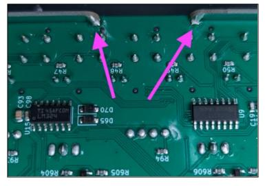
There are 2 small solder pads where the spacer PCB meets the main PCB, so you can solder the spacer PCB to the main PCB. For disassembly, the solder will have to be removed using a solder sucker or desoldering wick.
