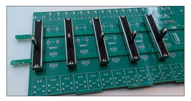
Now flip the PCB onto the side you just soldered the connectors to. Place the 2 edge rails you just snapped off across the PCB as shown in the picture. They will temporarily help set the height for the 5 slider pots (U21-U25). Put in those slider pots without soldering yet!
