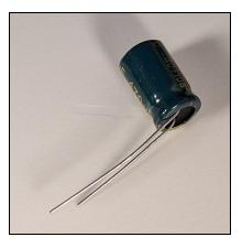
Insert capacitor C59 after bending its legs to the side. Scrooge is intended to produce the weirdest of noises, but the sound of an exploding capacitor should not be among them, so make absolutely sure to place it in the right orientation as shown in the picture!
