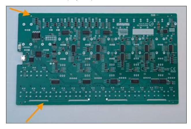
Use a pair of pliers to snap off the edge rails from the PCB. These are remnants from the manufacturing process. **Keep both edge rails for now, as you'll need them later in the build!**
