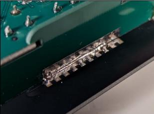
Now on to the remaining pads on the spacer PCB. The best way to solder them is to place the end of your solder wire across the pad as shown, and slowly move your (ideally very hot) soldering iron over it.
