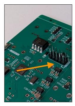
Insert the 10-pin Eurorack power header (J3) into the PCB footprint and solder from the other side.
