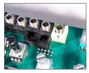
Then insert both LEDs. The long legs of the LEDs go on the side marked on the PCB with a "+". Double check the orientation! Put the small black LED housing on top as shown. The inside shape is tapered like a funnel: Make sure that the wider part is on top, and the open side points towards the sockets.
