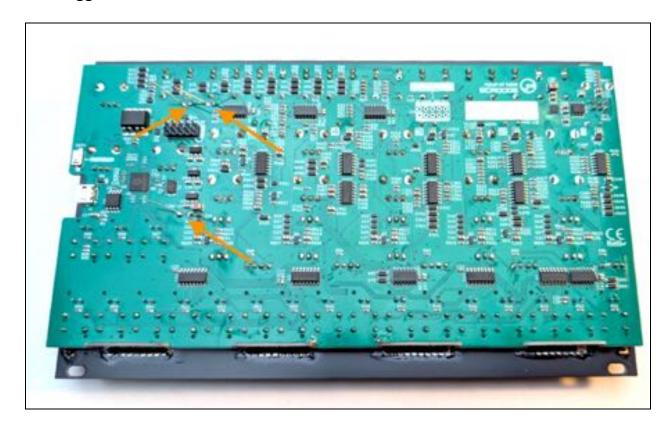
Now snip off the LED and capacitor legs with a wire cutter.
