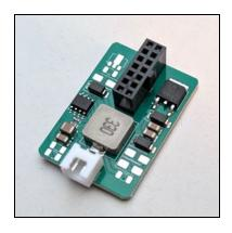
The desktop version has a small power supply module called PENNY A. It comes with 2 headers that are to be installed and soldered as shown in the image on the left. This module converts the 5V coming in via the desktop case's USB-C port to 12V, so it can be plugged into the Eurorack power connector. (Note that it does not generate -12V as this is not needed for Scrooge, so it will not power other Eurorack modules that need the
