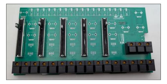
Pull the edge rails out to the side (they can be discarded now), remove the panel and insert the 19 buttons (SW11-SW29) into their footprints without soldering yet! They each have 2 plastic pins that need to sit securely in the holes on the PCB. Double and triple check the alignment of the buttons. It's best to look from all possible
