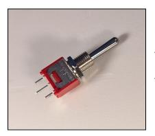
Each SPDT switch (SW1-SW10) has 2 nuts. Put 1 nut on each, all the way down the thread as shown in the picture. It doesn't have to be tightened. Put all the levers in the middle position. Now place all of the switches into their footprints on the PCB.
