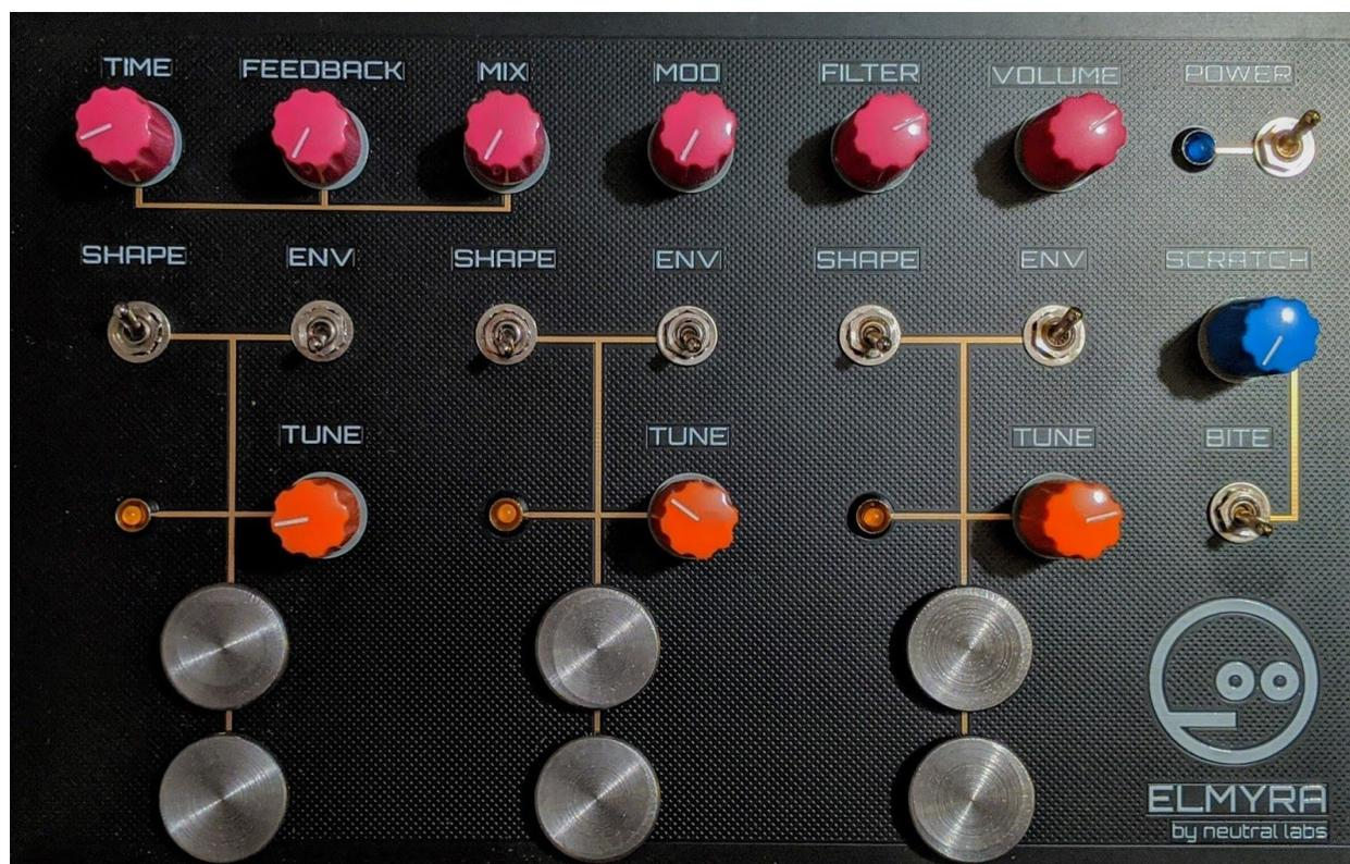
Elmyra's front panel has 3 sections: The voices (x3), the top row and the scratch/bite distortion circuit.
